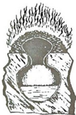
Figure 2.1. A Simple Illustration of the is simple illustration of the yantra for the downward distillation process
